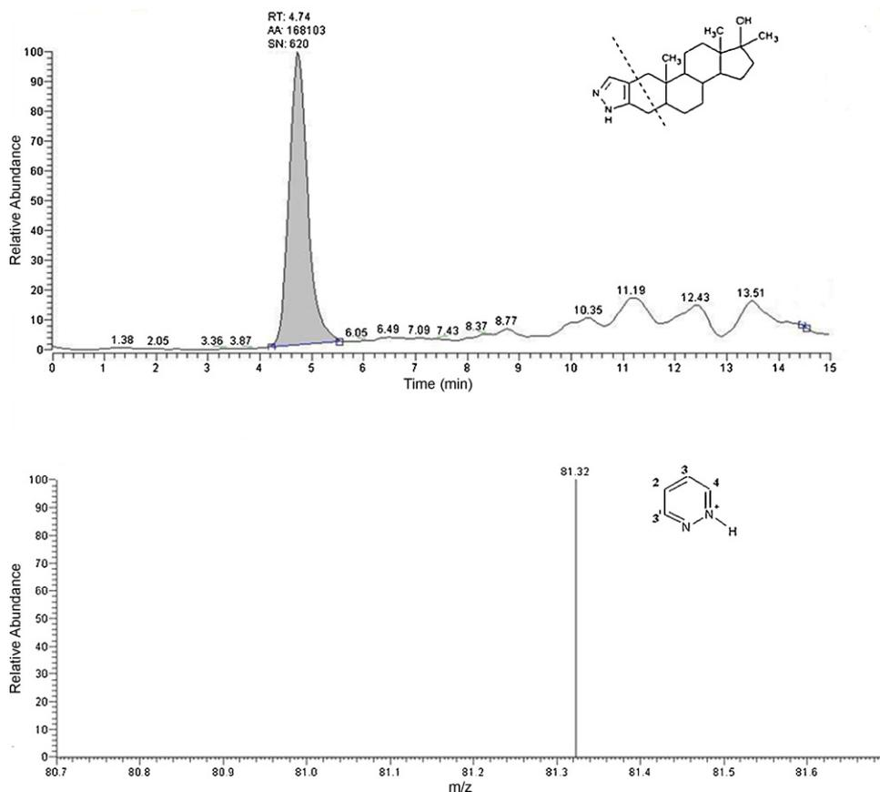
**Fig. 3.** LC–MS/MS chromatogram and CID spectra of stanozolol.
