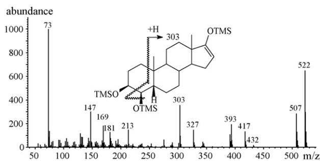
**Fig. 3 – Typical per-TMS mass spectrum of a 3,4-dihydroxy-5 $\beta$ -androstan-17-one (3 $\beta$ ,4 $\beta$ -dihydroxy-5 $\beta$ -androstan-17-one).**
