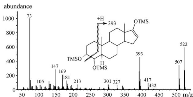
**Fig. 2 – Typical per-TMS mass spectrum of a 3,4-dihydroxy-5 $\alpha$ -androstan-17-one (3 $\alpha$ ,4 $\alpha$ -dihydroxy-5 $\alpha$ -androstan-17-one).**
