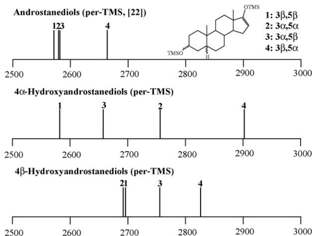
**Fig. 4 – Demonstration of retention indices of 3,4 $\alpha$ - and 3,4 $\beta$ -Dihydroxyandrostane-17-ones as per-TMS derivatives in comparison with retention of per-trimethylsilylated androstane diols.**
