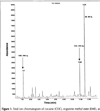
**Figure 1.** Total ion chromatogram of cocaine (COC), ecgonine methyl ester (EME), and benzoylecgonine (BE) in a plasma sample.
